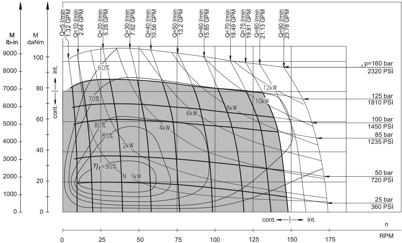
The function diagrams data is for average performance of randomly selected motors at back pressure 5÷10 bar [72.5÷145 PSI] and oil with viscosity of 32 mm<sup>2</sup>/s [150 SUS] at 50°C [122°F].
