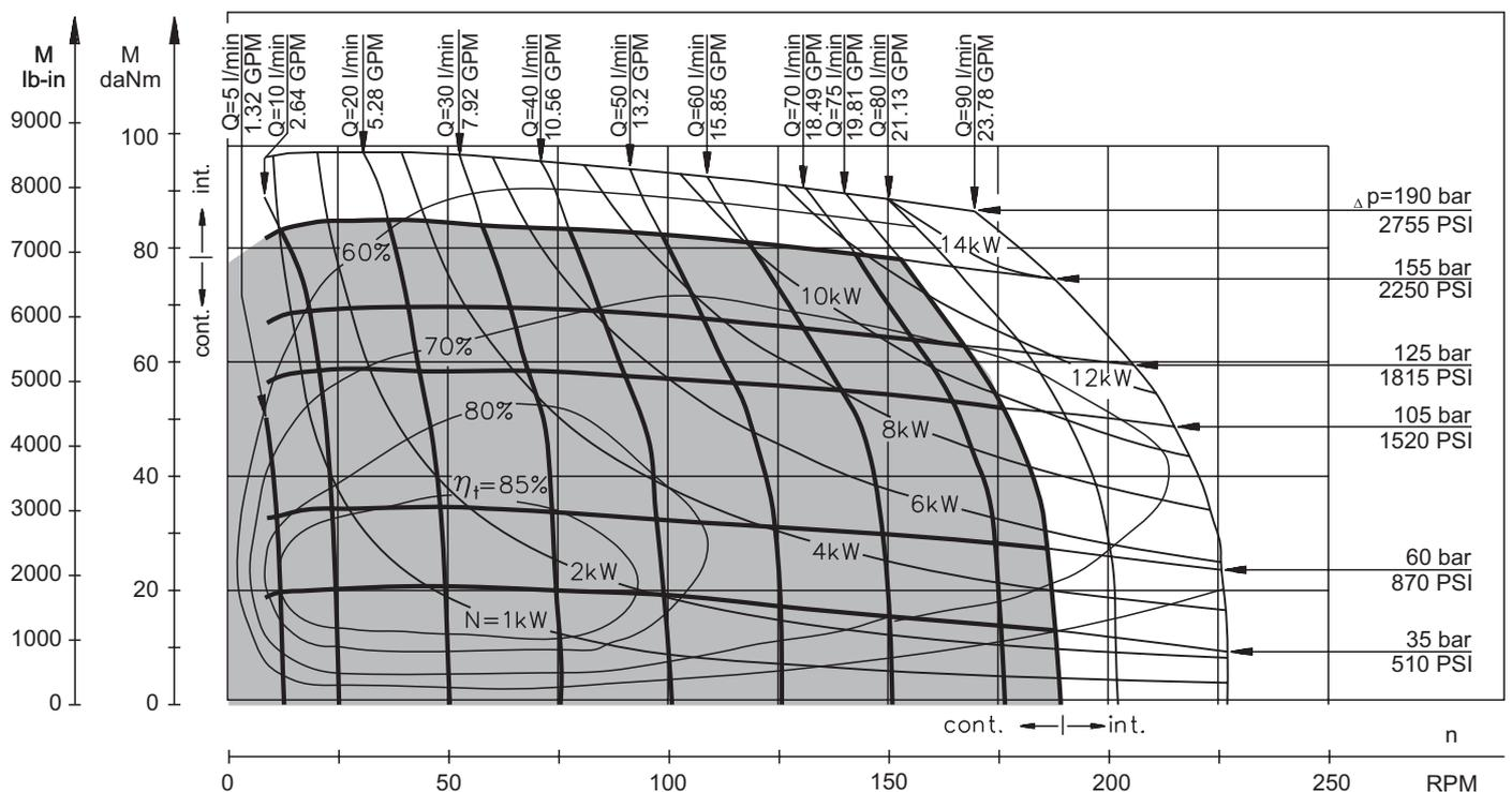
The function diagrams data is for average performance of randomly selected motors at back pressure 5 ÷ 10 bar [72.5 ÷ 145 PSI] and oil with viscosity of 32 mm<sup>2</sup>/s [150 SUS] at 50°C [122°F].
