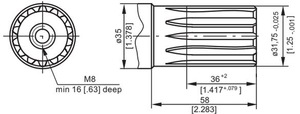
**CB** -  $\varnothing 35$  straight, Parallel key A10x8x45 DIN 6885
