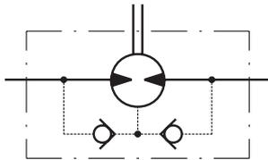
**MH... motors with standard shaft seal and with drain connection:**
