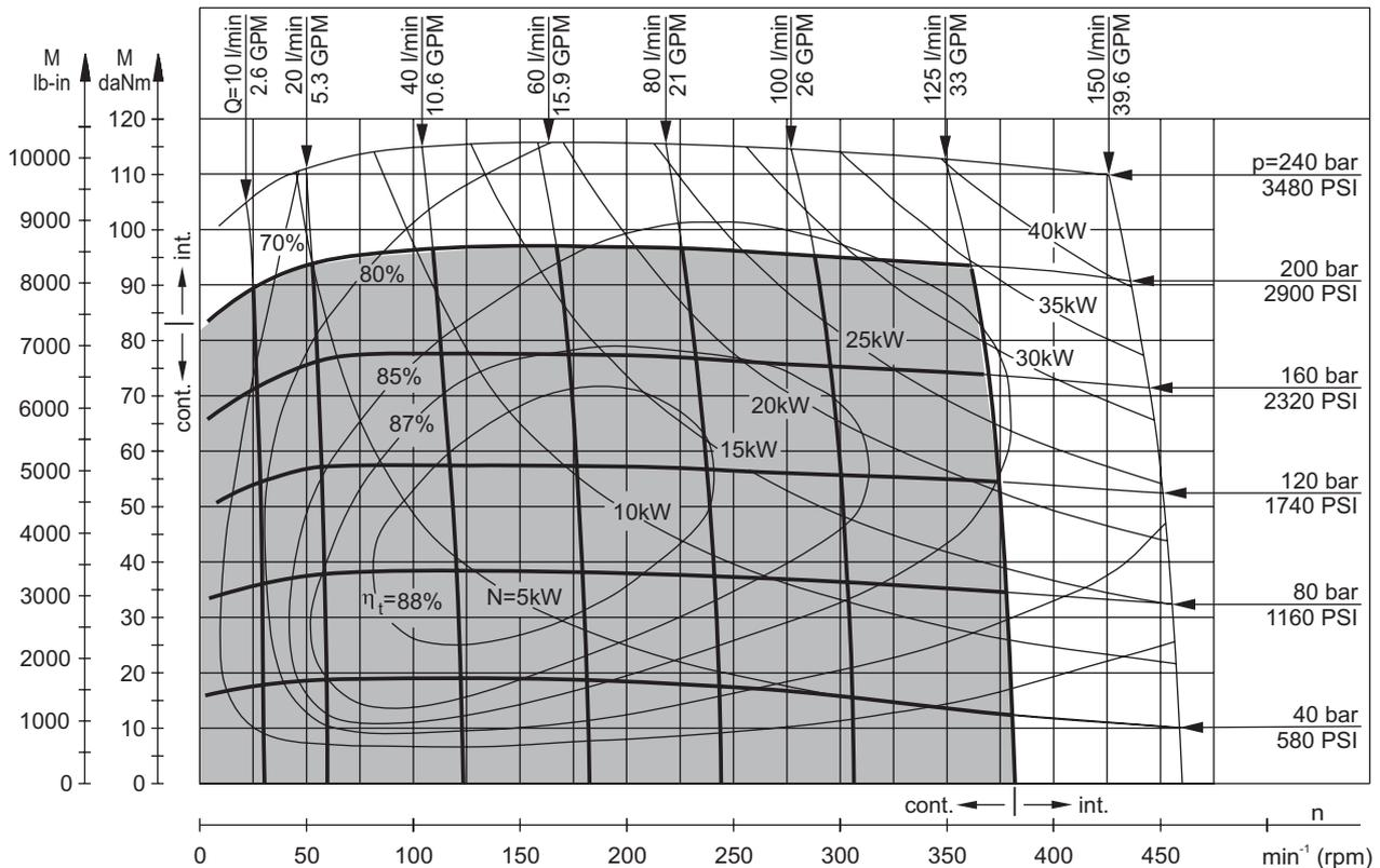
The function diagrams data is for average performance of randomly selected motors at back pressure 5÷10 bar [72.5÷145 PSI] and oil with viscosity of 32 mm<sup>2</sup>/s [150 SUS] at 50°C [122°F].
