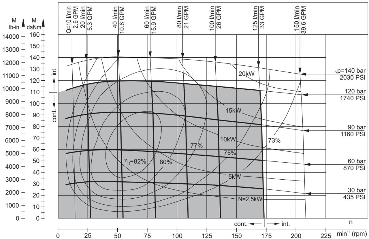
The function diagrams data is for average performance of randomly selected motors at back pressure  $5 \pm 10$  bar [72.5÷145 PSI] and oil with viscosity of 32 mm<sup>2</sup>/s [150 SUS] at 50°C [122°F].
