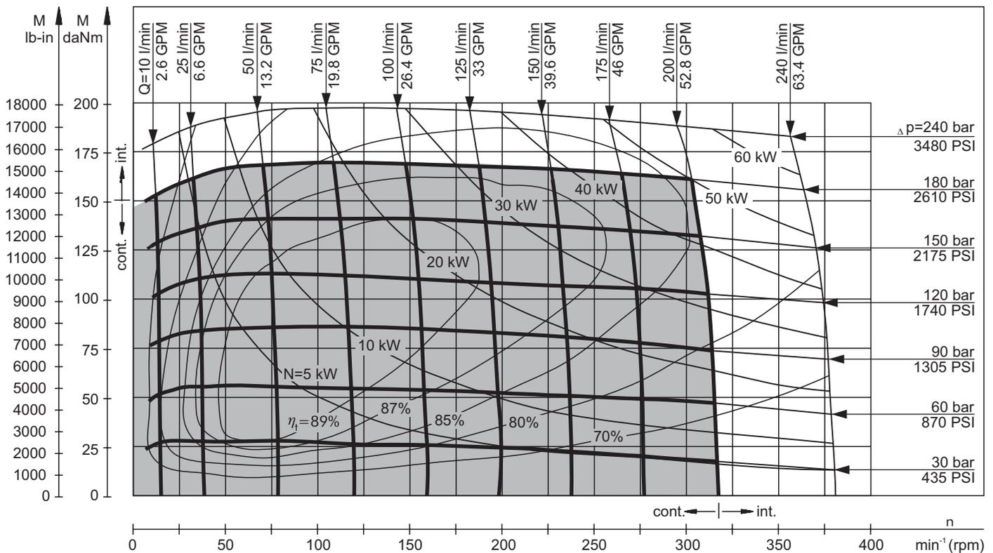
The function diagrams data is for average performance of randomly selected motors at back pressure 5÷10 bar [72.5÷145 PSI] and oil with viscosity of 32 mm<sup>2</sup>/s [150 SUS] at 50°C [122°F].
