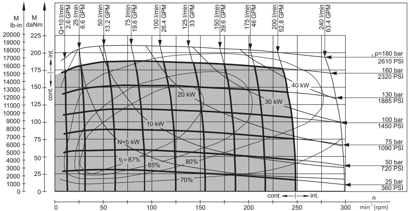
The function diagrams data is for average performance of randomly selected motors at back pressure  $5 \pm 10$  bar [72.5  $\pm$  145 PSI] and oil with viscosity of 32 mm<sup>2</sup>/s [150 SUS] at 50°C [122°F].
